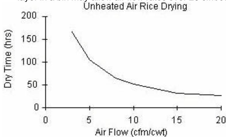
Figure 4. Effect of air flow rate on drying time for rice dried from 24% to 18% moisture with air temperature equal to September average for Red Bluff, CA.
