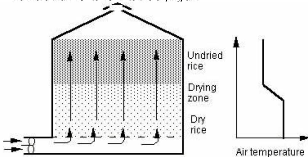
Figure 3. Air passing through a bed of rice produces a distinct drying zone.
